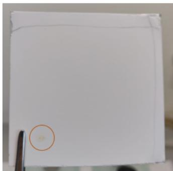
**Figure 3.4** Location of the initial spot of the industrial pitch sample on the TLC plate (6.5cm \* 6.5cm) for the 2D-TLC method (red circle)
