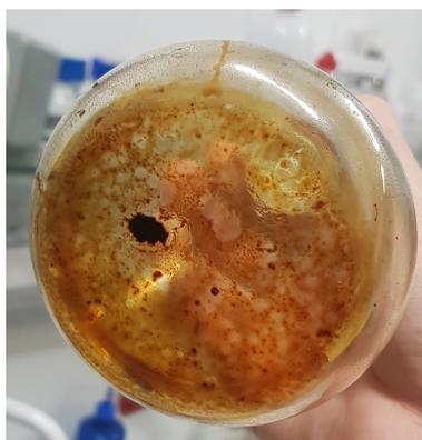
**Figure 3.1** Dried pitch sample from industrial paper mill
