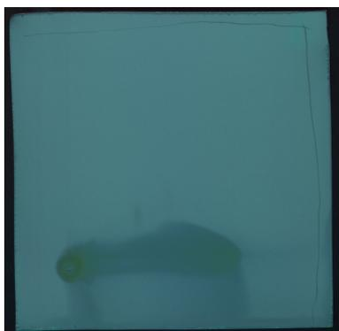
**Figure 3.8** Upper LOD: Overfilling of the initial spot with sample - Tailing effect
