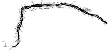
**Figure 2.7** Milled cellulose fiber with outer fibrils
