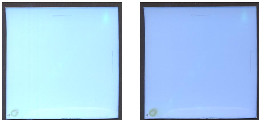
**Figure 4.8** Image from the first scan - scanning lamp not yet balanced (left); Image of the subsequent scanning process - intensity of the scanning lamp constant (right)
