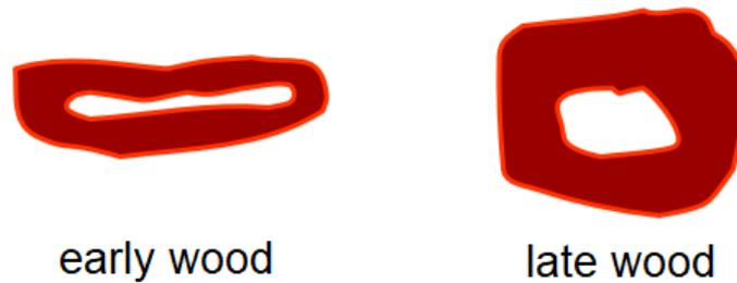
**Figure 2.11** Cross-section of early and late wood fibers
