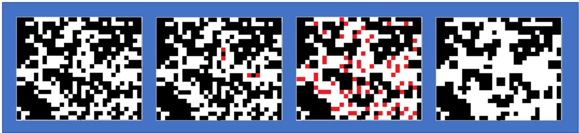
**Figure 3.12** Steps from the "PIXELKILL" function (Background: white pixel): Start picture (left); horizontal and vertical pixel detection (center-left); Elimination (center-right); Result (right)
