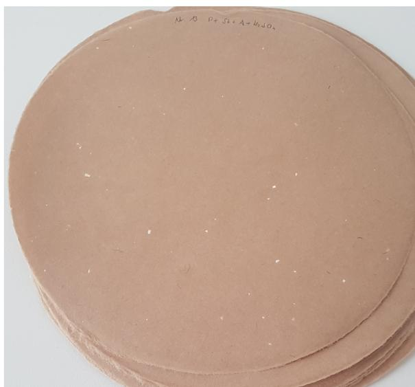
**Figure 3.3** Produced laboratory sheet with over 30 agglomeration stains
