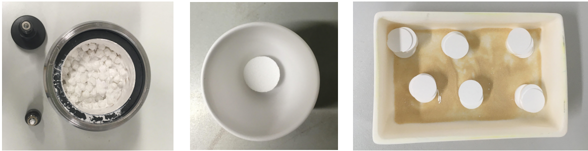
Figure 3.3: Stages of synthesis: ball milling (left), aggregation of powders after calcination (middle), pellets before sintering (right)
