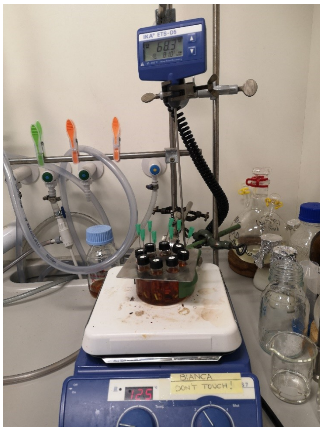
Figure 19 Multiple batch setup for Heck couplings (in the heat up phase)
