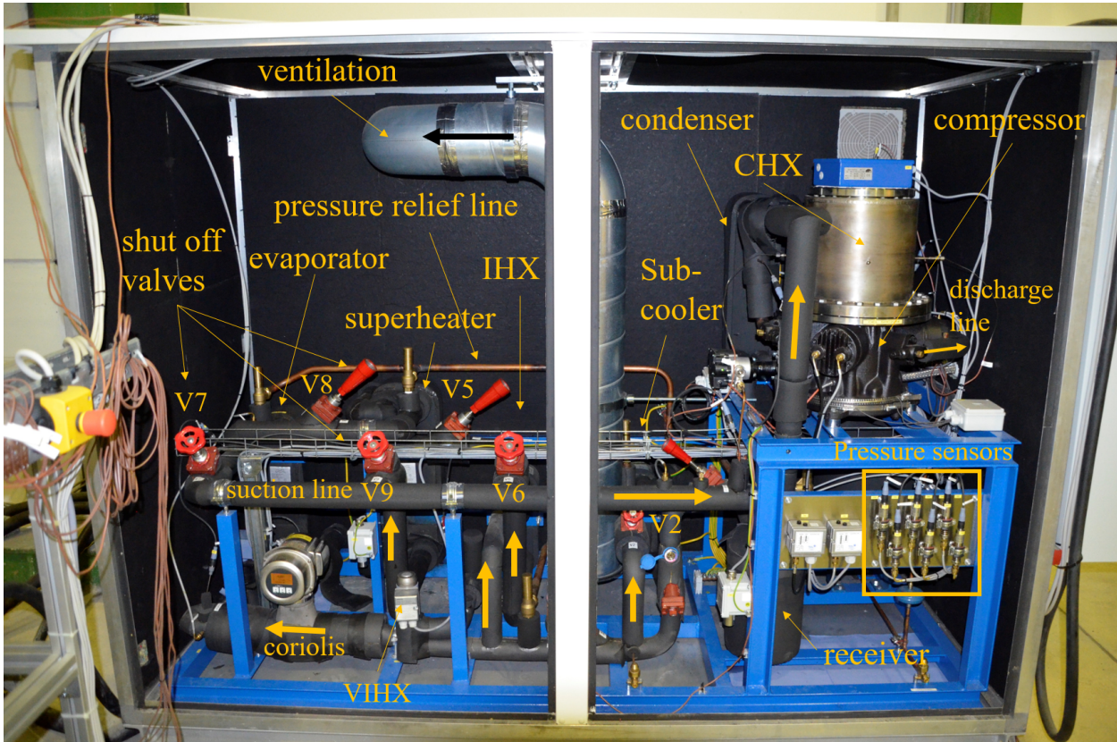
Figure 4.6: Front view of the R600 high temperature heat pump prototype with open housing, indicated flow directions and components
