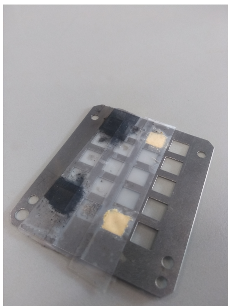
Figure 3.15: The inner part of the disassembled SAXS sample stage
