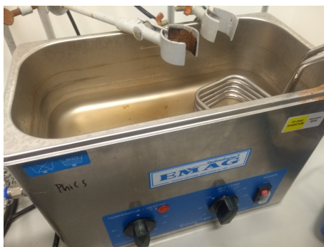
Figure 3.12: Setup of the sonication bath with external cooling coils
