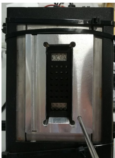
Figure 4.8: Chip in heating block - top view
