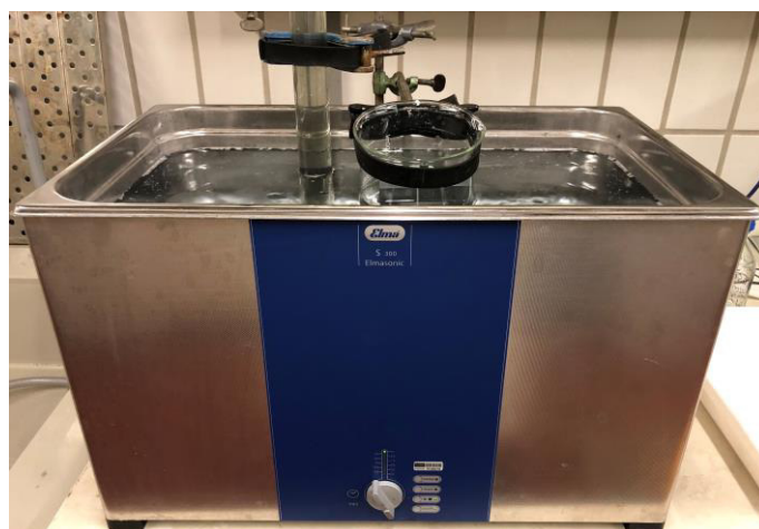
Figure 4.16: Ultrasonic bath with a beaker for complete impregnation of the support layer with membrane phase for the U-tube experiments.
