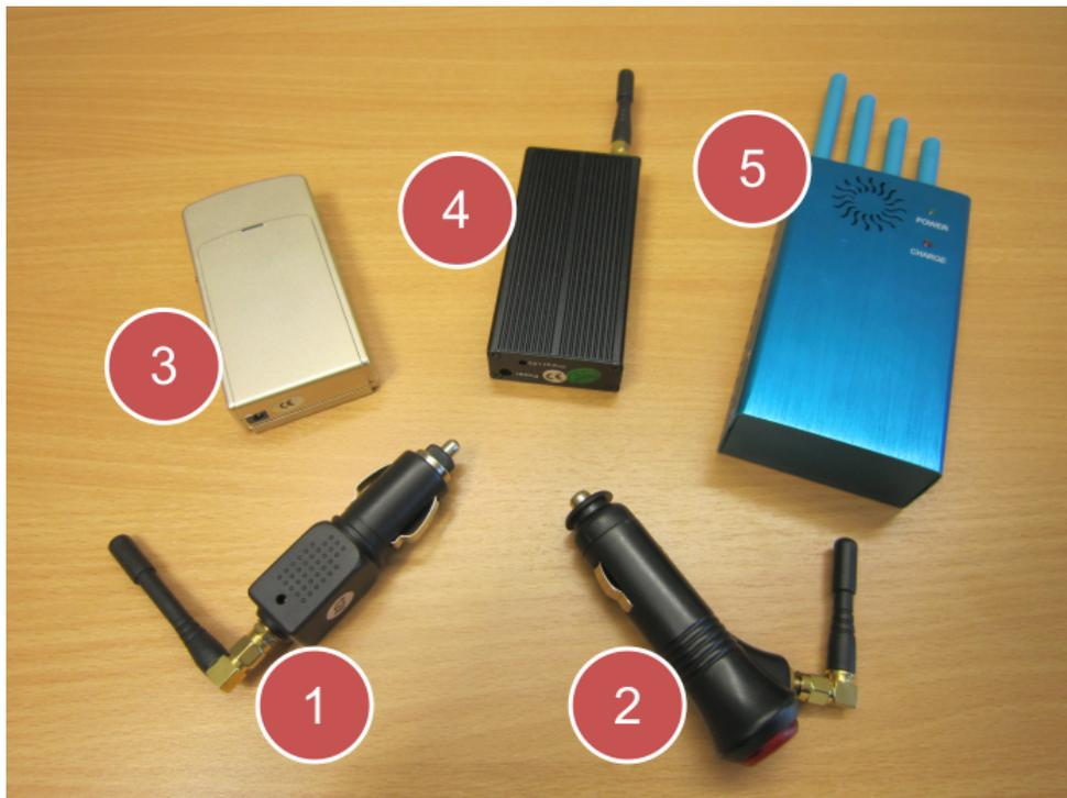
Figure 7.38: Jammers used for the test measurements
