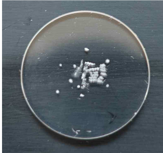
Figure 1.13: Damaged sapphire cover glass
