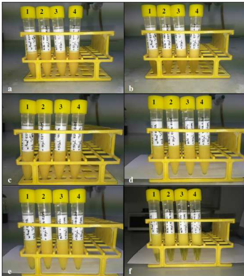
Figure 2.7: Optimization of milk emulsion preparation: effect of stabilizers, ultrasonic bath, and heating on emulsion stability and homogeneity. a After sample and reagents mixing and shaking. b Four minutes after shaking. c after sonication. d Twenty minutes after sonication e Forty-four minutes after sonication. f After 20 min of heating. 1 Without chemical stabilizer. 2 With EDTA. 3 With Triton X-100. 4 With EDTA and Triton X-100
