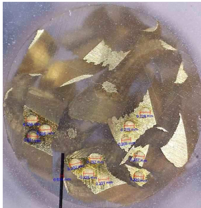
Figure 1.21: microscope picture of the sample BAM 229_a; digital determination of the crater diameters
