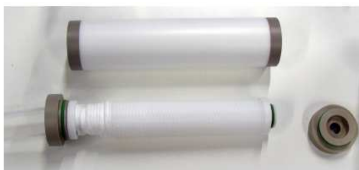
Figure 2.9: Picture of the assembled digestion tube coiled around the coil former, the PTFE outer tube and the PEEK end caps
