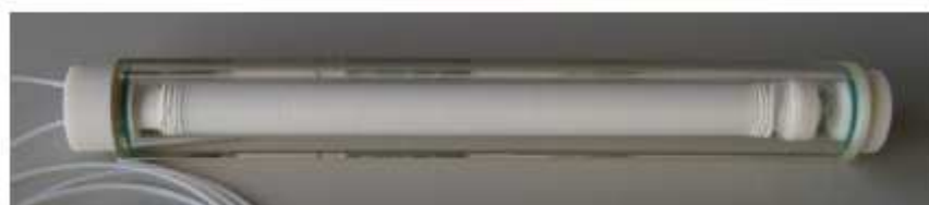
Figure 2.3: Picture of the glass tube reactor, including the coiled digestion tube and end caps
