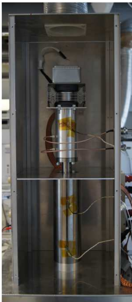
Figure 2.10: Upper part of the setup including the autoclave, launcher and magnetron
