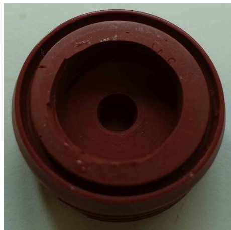
Figure 1.10: Negative silicon rubber form of the solid brass sample
