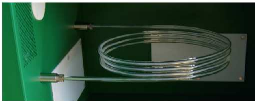
Figure 2.2: Glass coil reactor inside the Multiwave 3000 cavity
