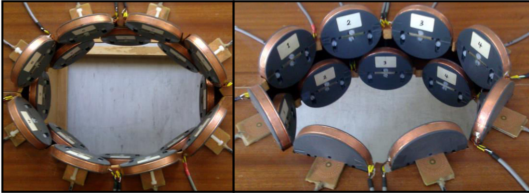
Figure (3.6): Configuration of the MITS transceiver array. Left: top view, right: three-dimensional (3D) view. A close-up view of the TRX is provided in figure (3.4).
