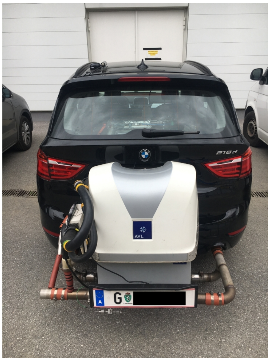
Figure 9: Vehicle with commercially available PN-PEMS (AVL MOVE) and DTT PEMS installed. Please click here to view a larger version of this figure.
