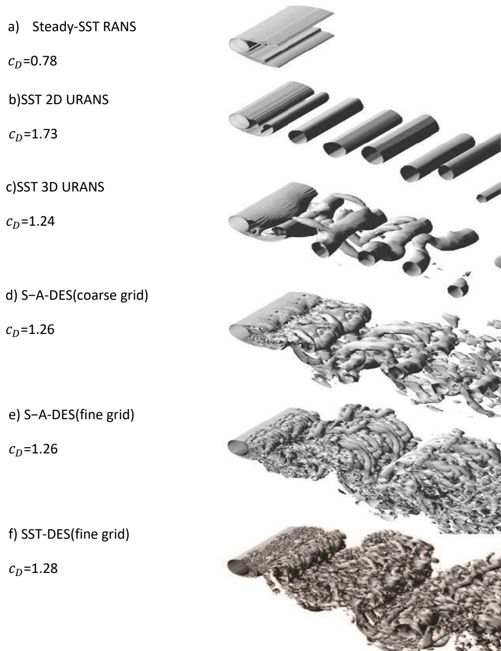
Figure 14: Flow around a circular cylinder with visualized isosurfaces of vorticity[13] Re=5 \times 10^4 .
