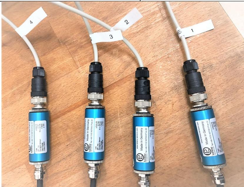
Figure 47: Charge amplifiers with paired sensor- and connection cables
