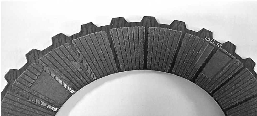
Figure 16: Defective Friction Plate because of Gauges
