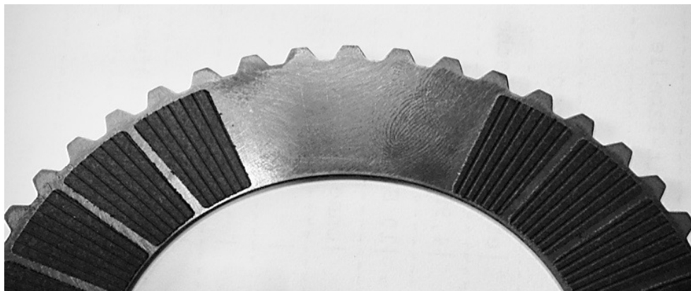
Figure 14: Defective Friction Plate because of Missing Segments
