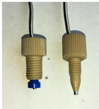
**Figure 3.23:** Right: First the conical HPLC fittings were used which generated a dead volume. Left: The new flat bottom fittings have an additional ferrule as sealing, which eliminated the dead volume.
