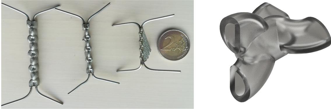
**Figure 3.1:** Left: The size-scaled-mixers have the same design, but their dimensions are scaled with factors of 0.75 and 0.5 referred to the large version. Right: Rendered image of the mixing structure consisting of two semi-circles between each mixing chamber.
