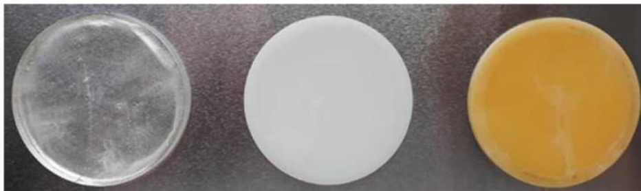
Figure 16: Photography of test specimen of the different epoxy resins. Left: Epoxy Resin 1, middle: Epoxy Resin 2, right: Epoxy Resin 3. The diameter of the specimens is d = 50 mm.
