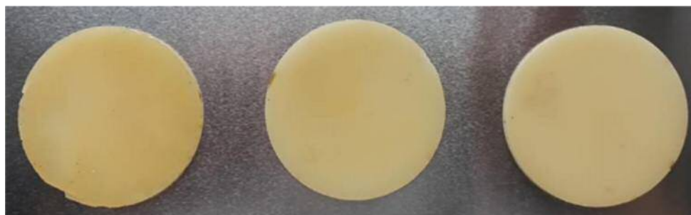
Figure 18: Test specimen of the different poly(2-oxazoline)s. Left: Polyoxazoline 1, middle: Polyoxazoline 2, right: Polyoxazoline 3. The diameter of the specimens is d = 50 mm.
