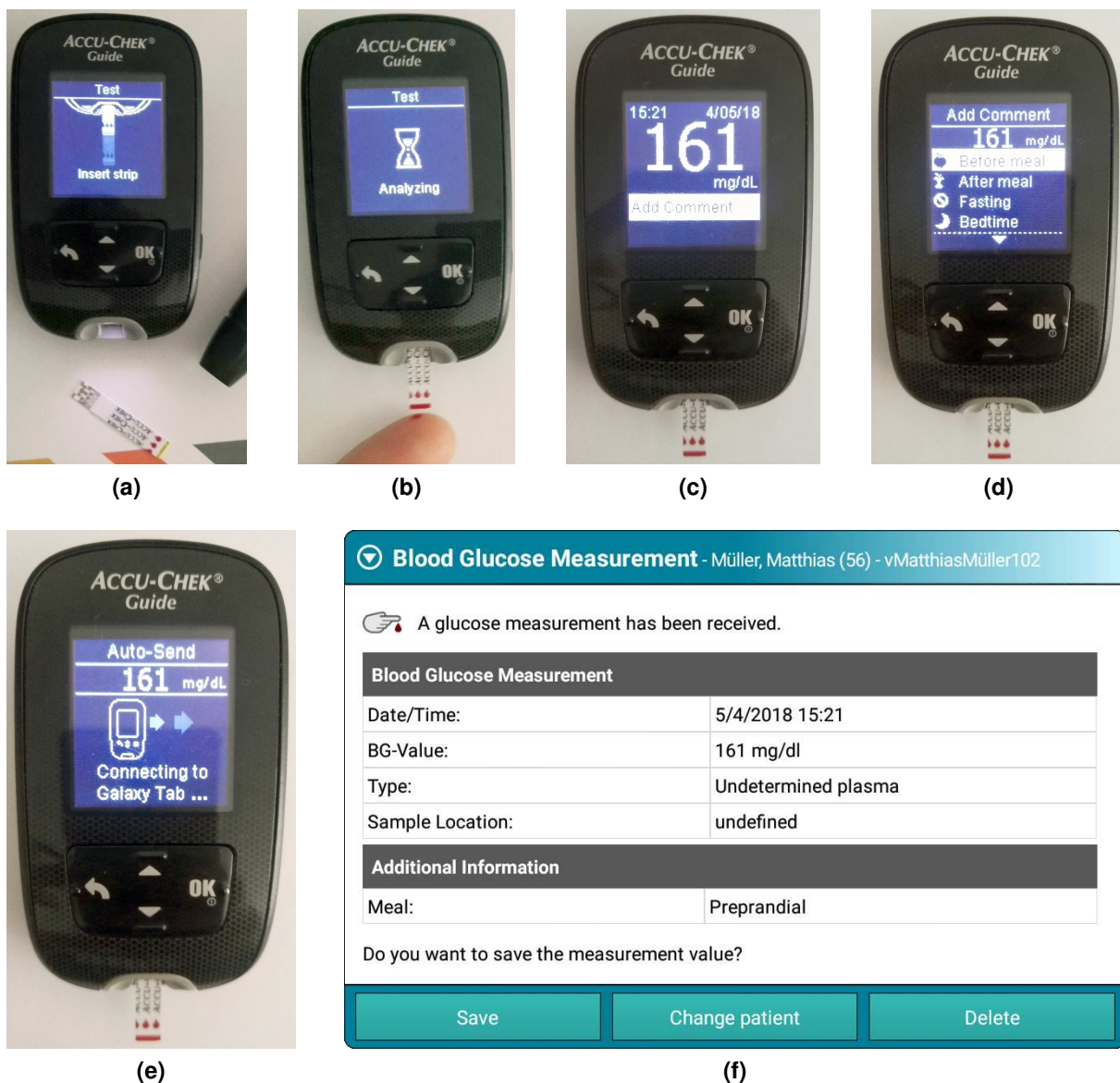
Figure 7.8: Workflow of performing (a, b) and annotating (c, d) a glucose measurement followed by an automated glucose measurement transmission to GlucoTab@MobileCare (e, f).
