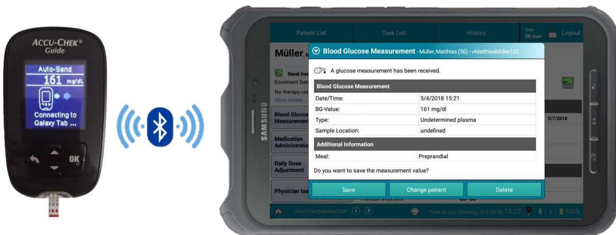
Figure 7.6: Automated glucose measurement transmission from an Accu-Chek® Guide glucose meter to the GlucoTab@MobileCare Android application.
