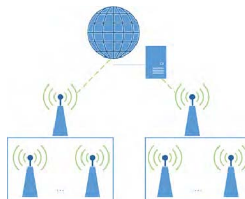
Fig. 3. The network structure in RESCATAME consists of two networks, where the 10 and 25 node send the sensor data to a router, that sends the data to a server.
