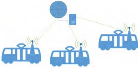
Fig. 6. In OpenSense, data measured by the tram-mounted nodes, are transferred to the server via GSM or WiFi.
