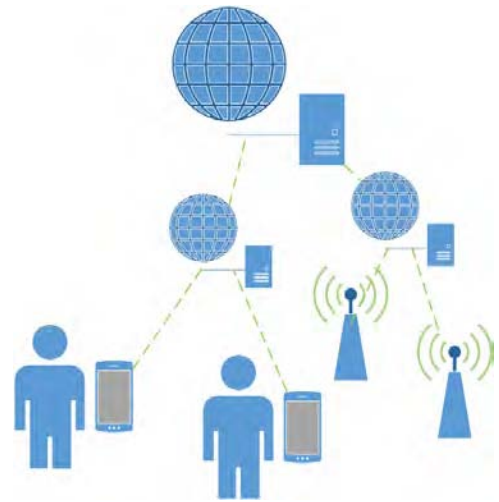
Fig. 5. In CITI-SENSE, fixed nodes send data to a server via GPRS/UMTS. Mobile nodes send data to a smartphone via Bluetooth which sends the data to a server.
