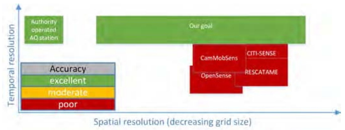
Fig. 7. The goal of our project in terms of sensor-accuracy, and spatial and temporal resolution.
