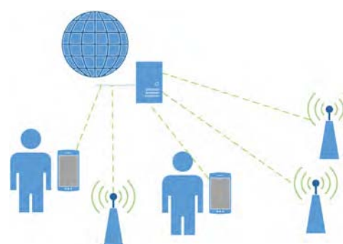
Fig. 4. In CamMobSens mobile and fixed nodes send data to a server via GPRS modules.
