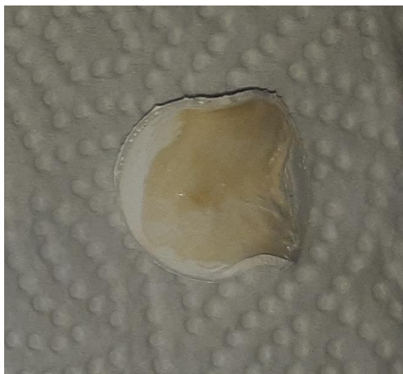
Figure 31: deformed disk deswollen after swelling in toluene
