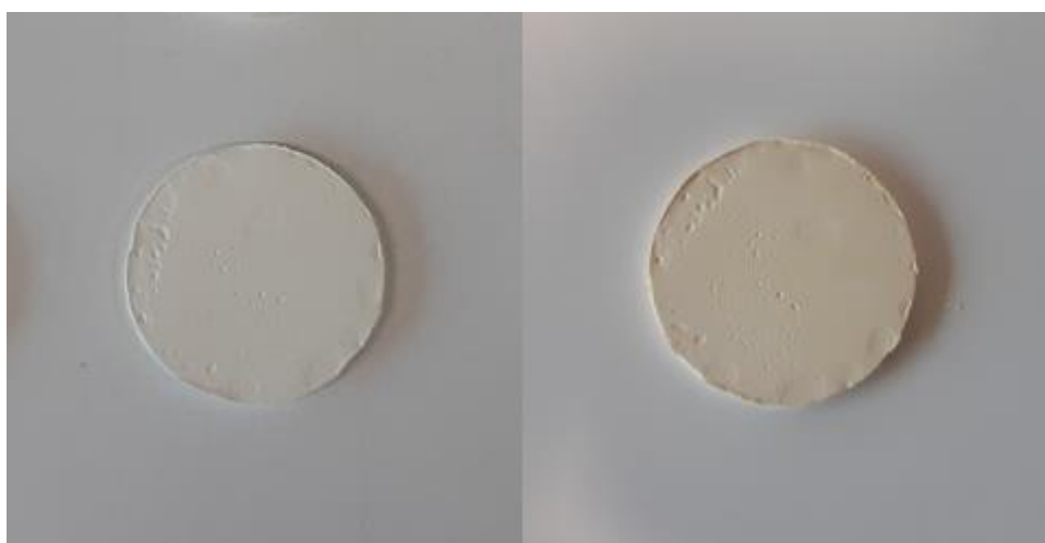
Figure 33: polyHIPE disk before (left) and after oxidation (right)
