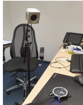
Fig. 8: RIR recording setup using a 5W measurement loudspeaker and a 6-channel microphone array [60].
