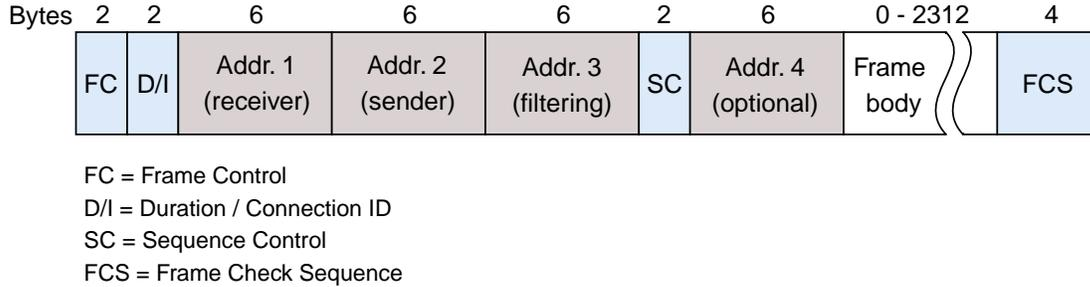
Figure 4.3: *Generic IEEE 802.11 data frame format*. The FC field defines the frame type; the number and function of MAC addresses depends on the deployed network type. The frame body can have a maximum size of 2312 bytes and after that a 32 bit CRC is added in the FCS field [77, 78].
