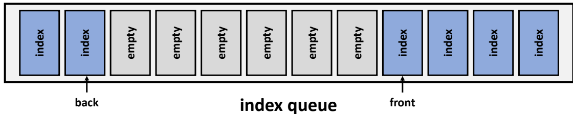
Figure 4.3: Both vertices and pages can be re-used by utilizing an index queue to keep track of the freed indices. This queue is array-based, built on top of a ring buffer using a front and back pointer (index) of static size.
