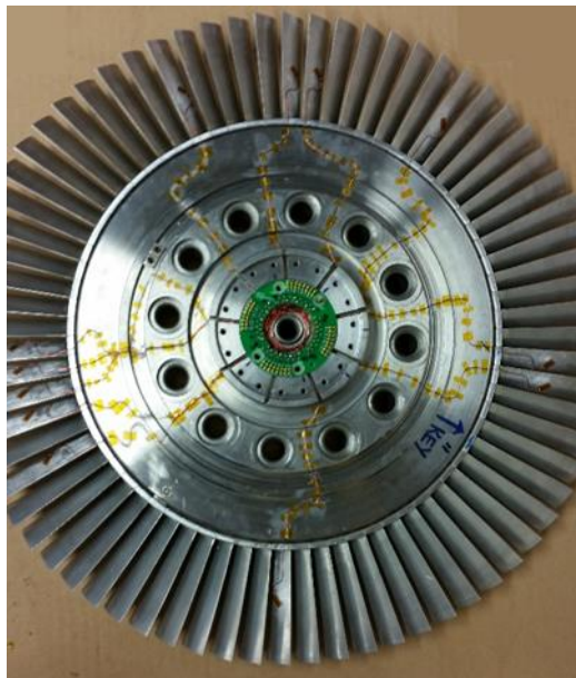
FIGURE 5.15: Rotor instrumented with strain gauges and circuit connection board.
