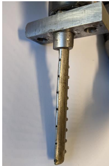
FIGURE 4.11: Injector rake for air injection in plane 0
