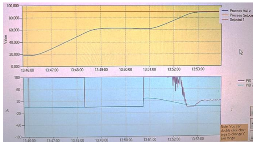
FIGURE 4.15: Screenshot of the temperature control software. Upper plot: air temperature (blue) and set-point (orange). Lower plot: graph of the PID regulation output (purple).
