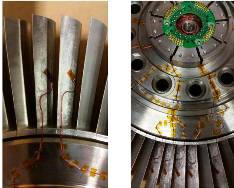
FIGURE 5.16: Photos of the rotor blades and disc during the instrumentation process.
