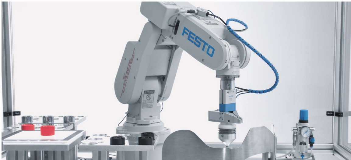
Figure 2.4: Articulated robot, online source [27.09.2020].
