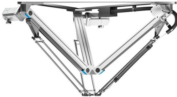
Figure 2.6: Parallel kinematic delta robot, online source [27.09.2020]
