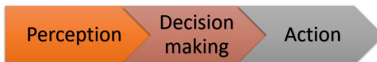
Figure 2.8: The sequence of steps that a robotic system undergoes to perform an action, Source: own illustration.
