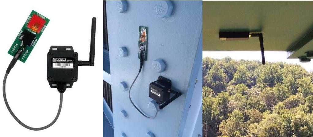
Figure 1.1: Wireless strain gauge from Resensys [1] mounted on a bridge.
