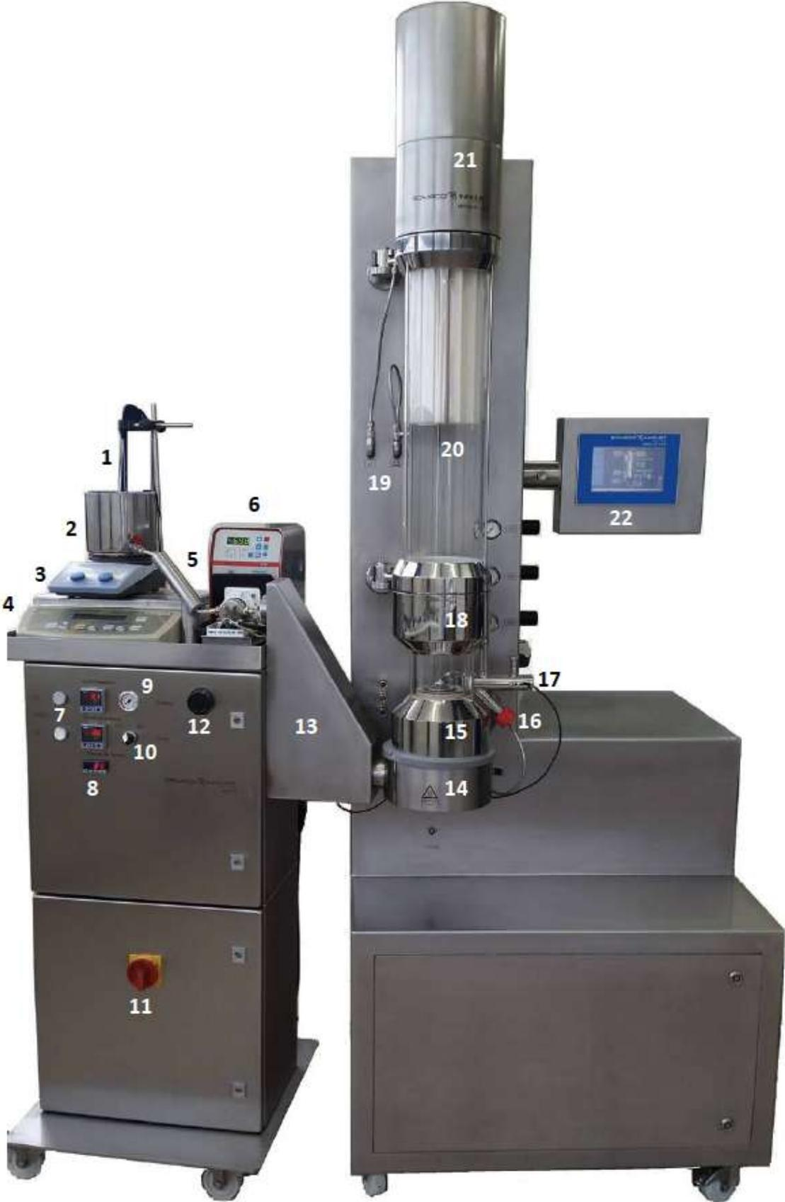
Figure 13 Innojet Ventilus V-2.5/1 with IHD Hot Melt Device (Becker K. , 2016)
