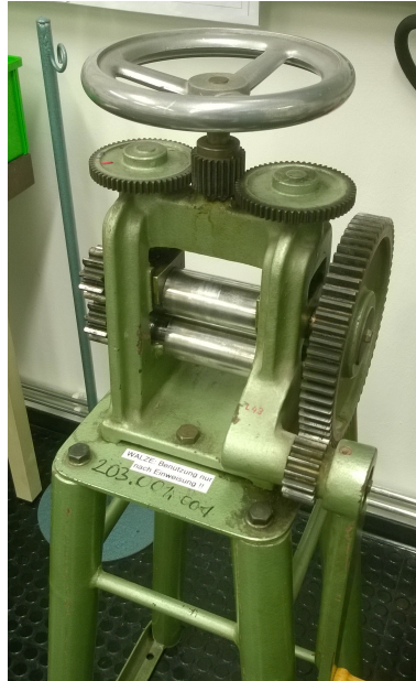
Figure 4.1.2: Cylindric roll used for the deformation of the samples.
