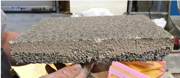
Abb. 3-9: Substratbeton
