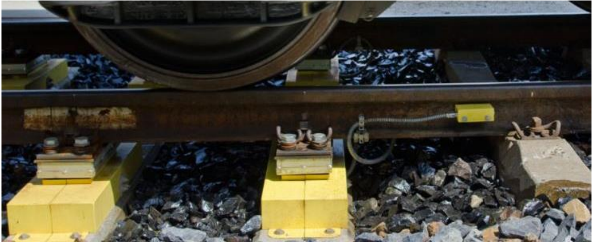
Figure 3-14 - Force sensors built into the sleepers.
