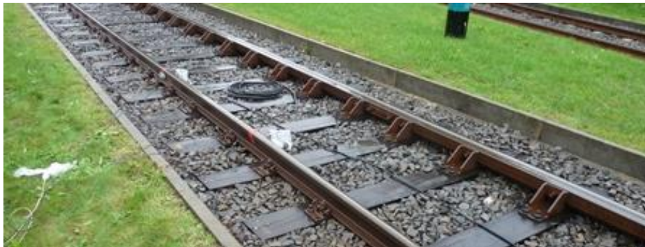
Figure 3-24 - Array of sensors measuring the structure-borne noise in the rail. Source: [76].
