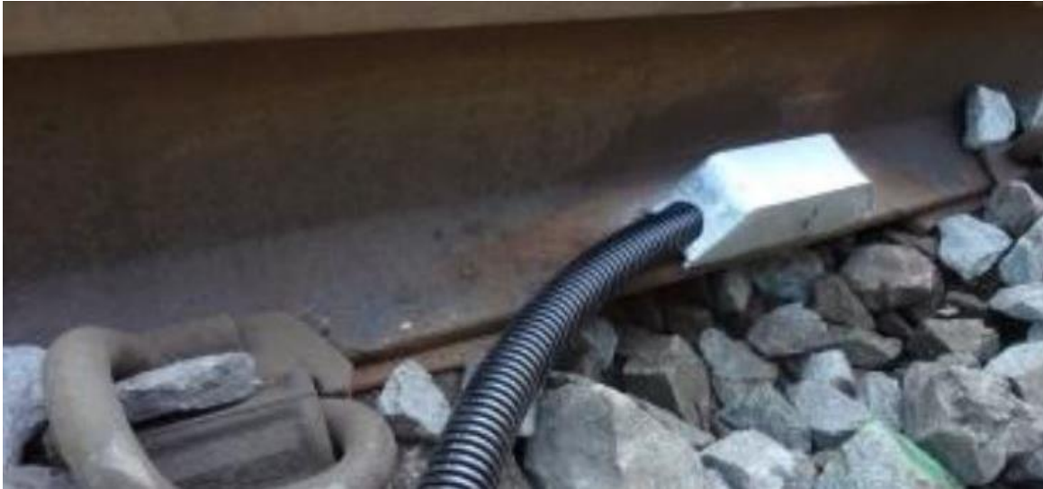
Figure 3-20 - Acceleration sensors glued to the rail. Source: [70].
