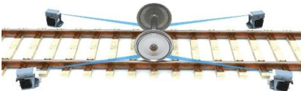
Figure 3-8 - Visualizing the working principle of MERMEC W-Inspect. Source: [55].
