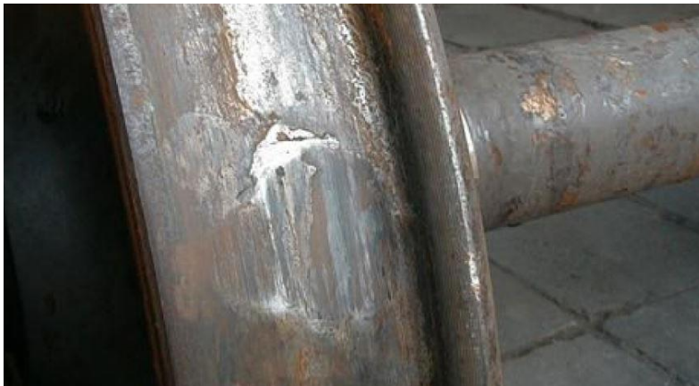
Figure 2-4 - Wheel flat with a subsequent material deposit. Source: [22].
