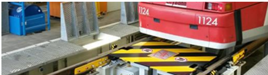
Figure 3-23 - Automatic measurement system. Source: [73].
