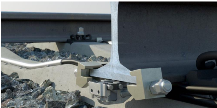
Figure 3-16 - Clamped on optical Sensors: Source: [64].
