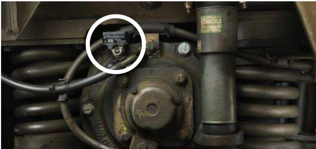
Figure 3-19 - SKF monitoring system Insight Rail mounted on the axle box bearing. Source: [69].
