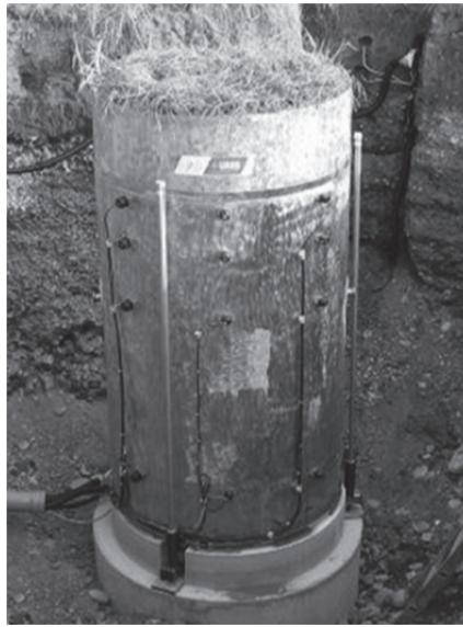
Fig. 64: Grass-covered Lysimeter in the testfield “Wagna” in Austria (Fank & Unold 2007, adapted)
