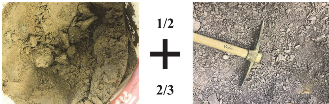
Fig. 41: (Left) “silty sand” (right) “compacted slate”
