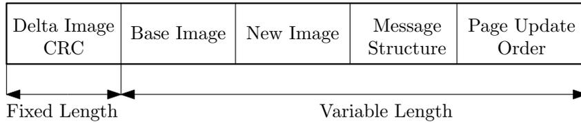
Figure 3.10: Delta Image Header Structure.
