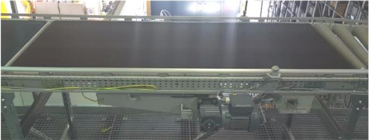
Figure 2-21: Belt conveyor with rigid support 2m (Lottersberger & Hafner, 2016)
