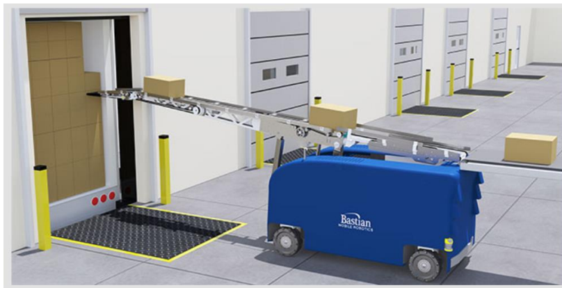
Figure 4-51: Robot for automated loading/unloading of trucks [BAST19]
