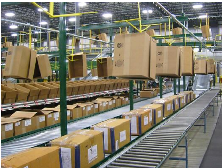
Figure 4-49: Overhead conveyors [PAC19]
