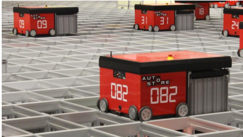
Figure 4-42: AutoStore robots [IXT19]
