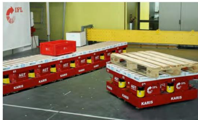
Figure 4-55: Small autonomous vehicles in the KARIS PRO System [HK14]
