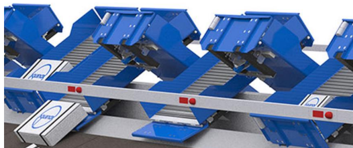
Figure 4-57: Slide tray sorter [EQU19]
