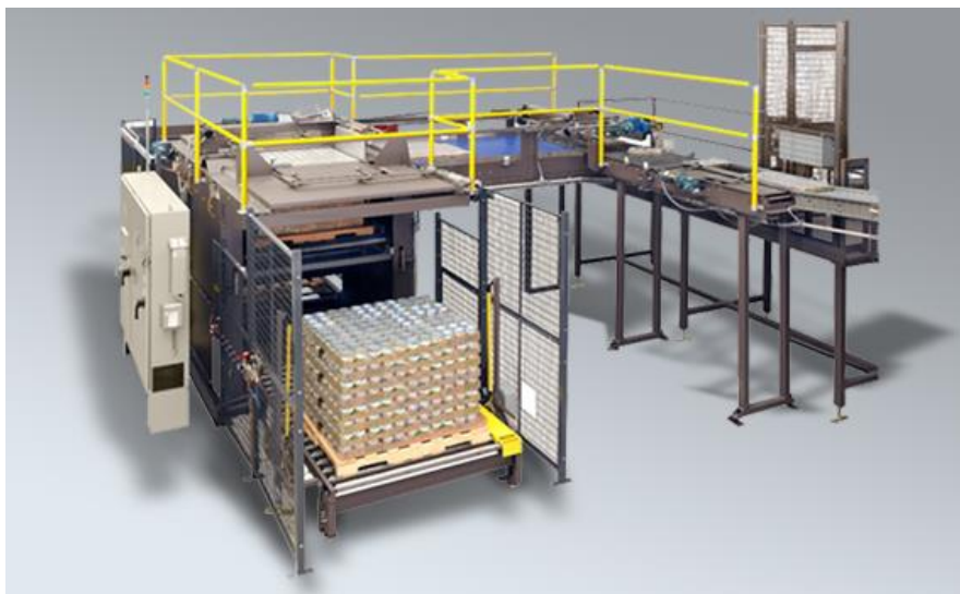
Figure 4-34: Conventional stripper plate palletizer [AMP19]
