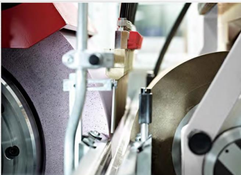
Figure 2.14: Centreless grinding machine, Online source: www.mikrosa.com [26.04.2019]
