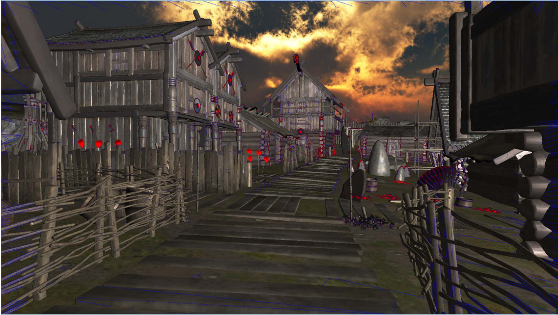
Figure 6.1: Visualizing high density hot spots of triangles per pixel where spatial aliasing occurs due to primitives missed in standard visibility sampling (marked in red). Our method can detect small triangles within these areas to include them in the visible set.
