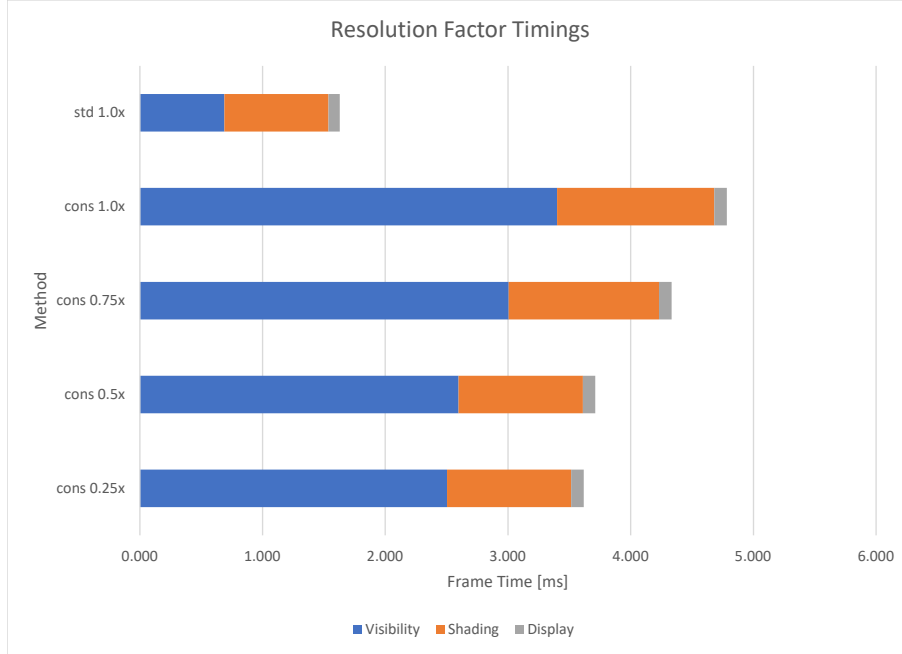
Figure 6.10: Frame times of the conservative visibility in various resolutions compared to standard sampling. Again, cons is our method using conservative visibility, std is standard sampling. 0.5x etc indicates the proportional resolution (e.g., 0.5 \cdot 1920 \times 1080 = 960 \times 540 )
