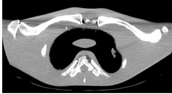
Figure 2.6: CT image of a shoulder phantom shows streaking artifacts caused by photon starvation [34].
