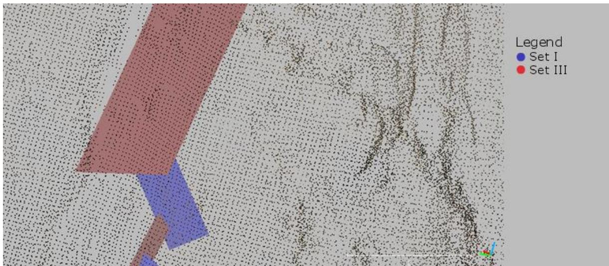
Figure 125: Fracture pattern of set I and III in detail over the RGB point cloud, left border of the big magenta plane in the figures above. Software used: CloudCompare (2019).
