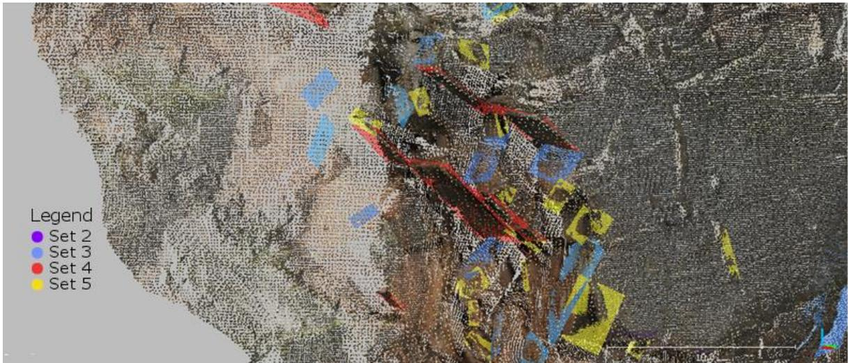
Figure 32: Fracture pattern in detail over the RGB point cloud from the left (from viewer's point of view), without set 1. Software used: CloudCompare (2019).
