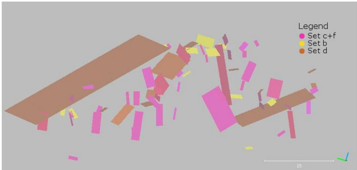
Figure 66: Fracture pattern in frontal view, without set a. Software used: CloudCompare (2019).
