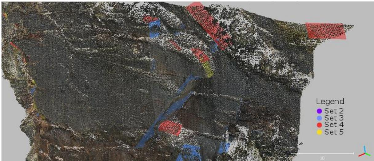
Figure 33: Fracture pattern in detail over the RGB point cloud from the right (from viewer's point of view), without set 1. Software used: CloudCompare (2019).
