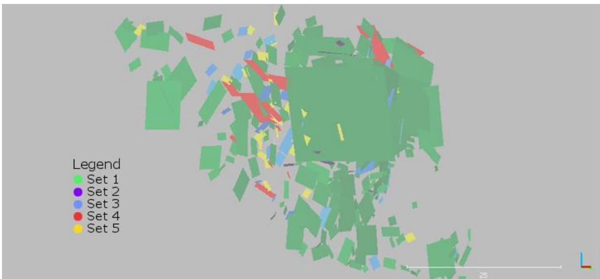
Figure 27: Fracture pattern in side view (left side from viewer's point). Software used: CloudCompare (2019).
