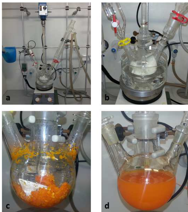
Figure S2. Overview on the xanthation of alkali cellulose. a: Preparation of the xanthation apparatus with the alkali cellulose deposited in the flask, b: Start of xanthation by adding CS 2 dropwise, c: Cellulose xanthate after 3 hours of stirring, d: Final viscose solution
