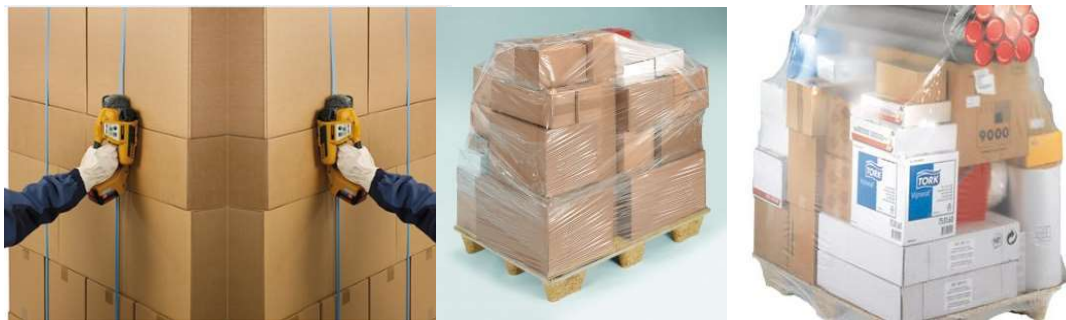
figure 15: load securing techniques of strapping [RAJ19b], stretching [RAJ19c], and shrinking [RAJ19d]
