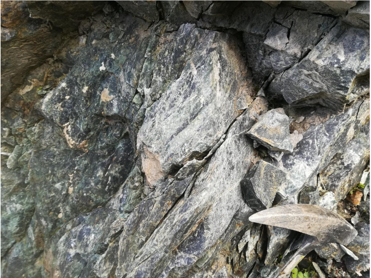
Figure 6-4: Strongly jointed, dark-greenish to grey greenish serpentinite in the central part of the study area.
