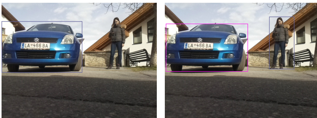
Figure 5.5: Car and Person inference with SSD Mobilenet V1 Coco network Figure 5.6: Car and Person inference with assistant system network
