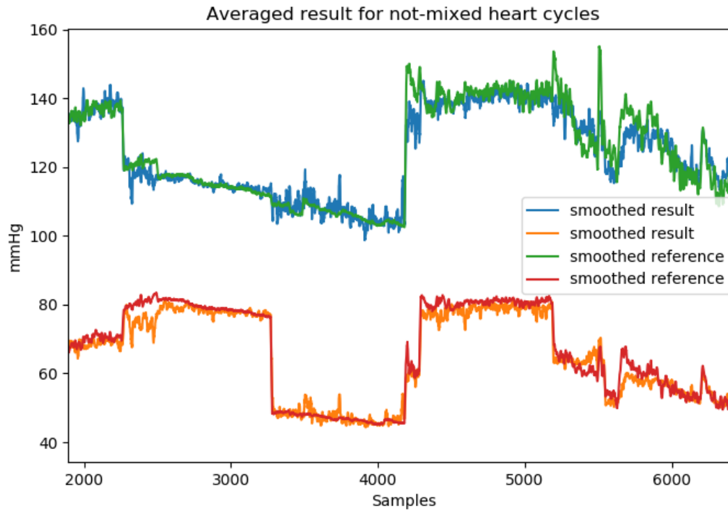
Figure 5.4.: Estimated and invasive measured systolic and diastolic blood pressure values of the testing data in mmHg; Final result for database data by using over 500.000 heart cycles from 56 test persons for training and 150000 cycles for testing; Averaged heart periods over 10 cycles in chronological order; For averaging a moving average filter was applied, the resulting edges were cut off; Measurements of different persons were lined up (Zoom 5.3)
