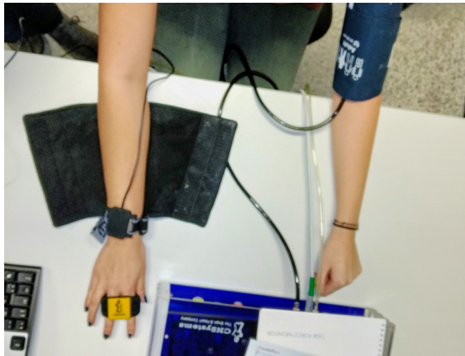
Figure 4.5.: Measurement setup; Left arm: Task Force Monitor finger-cuff and PALS-2 demo board; Right arm: Task Force Monitor arm-cuff
