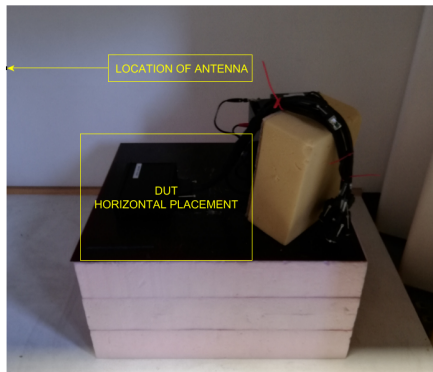
(a) Horizontally placed DUT in a chamber
