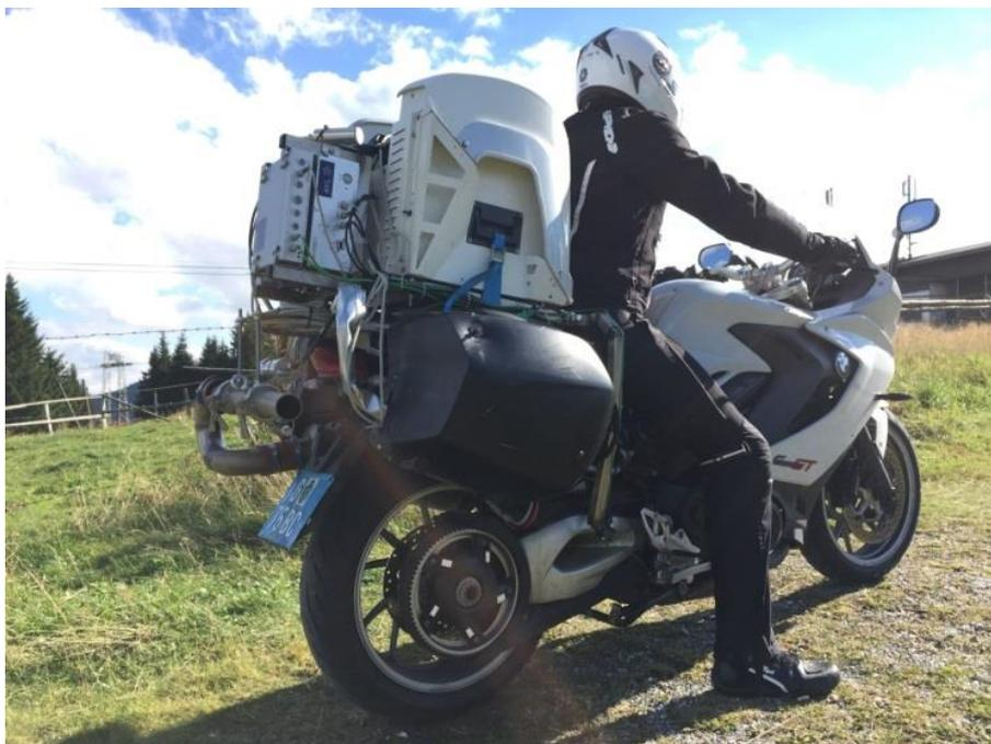
*Figure 24. Fully equipped BMW F800 for RDE and GPS measurement.*
