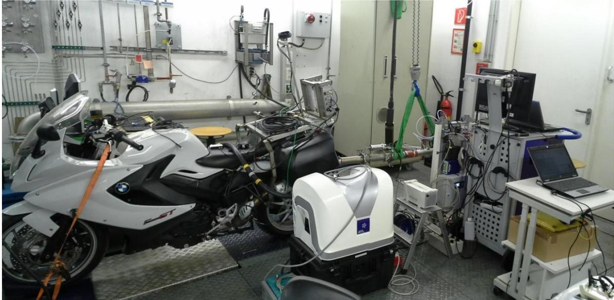
*Figure 19: Chassis dynamometer with additional measurement equipment for cross checks.*
