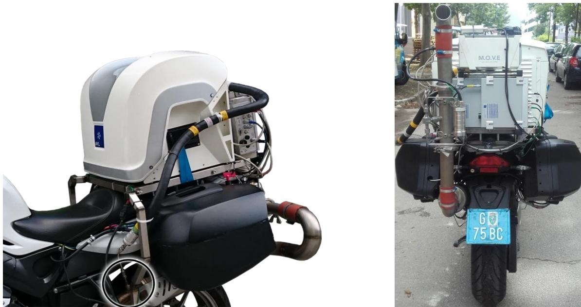
*Figure 17. Detailed view of PEMS and exhaust gas tapping position, left-hand side. Former vertical mounting position of the EFM, right-hand side.*
