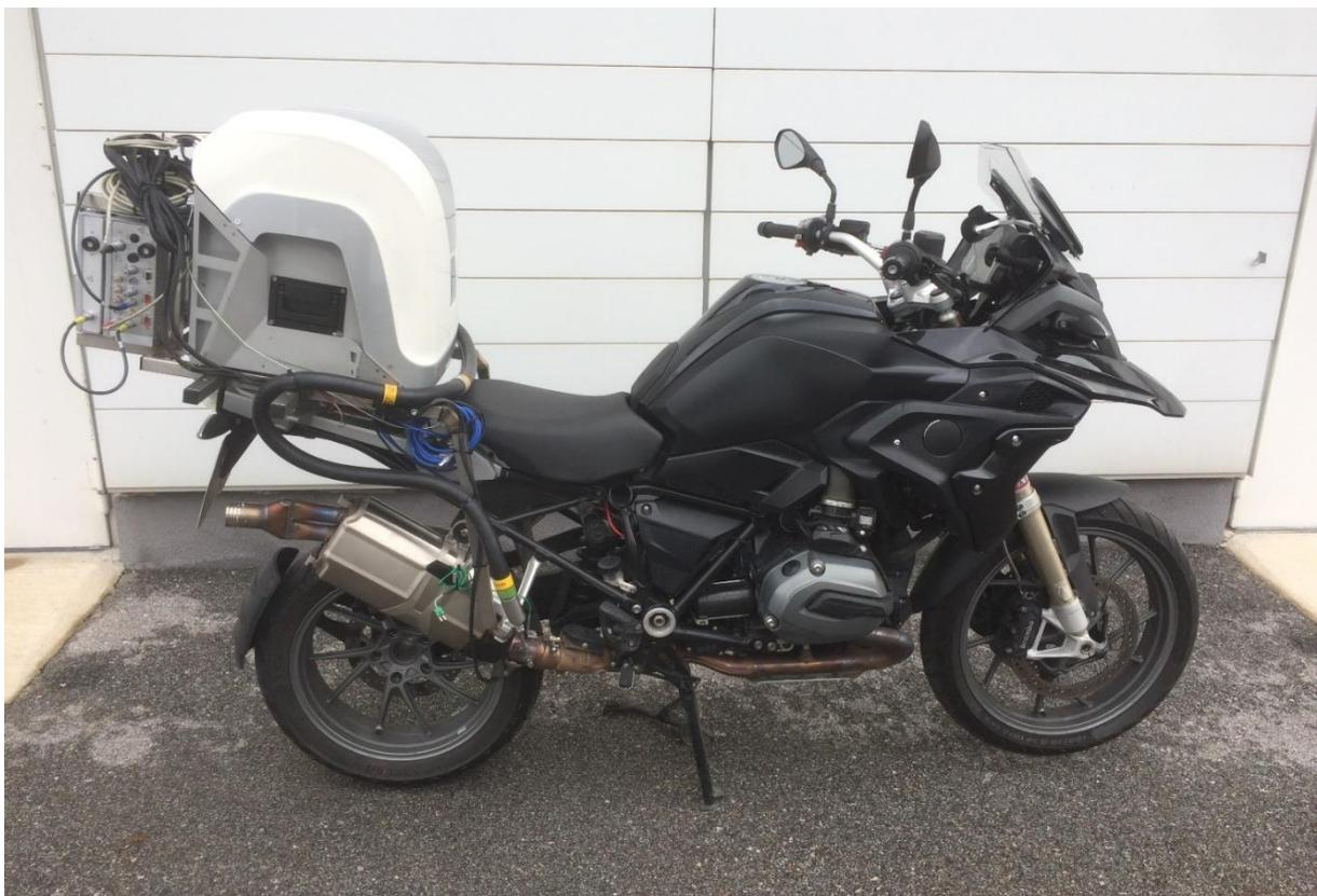
*Figure 110: Full PEMS equipment mounted on a BMW G1200GS motorcycle.*
