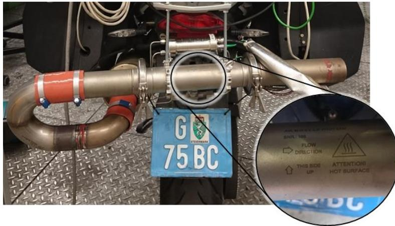
Figure 28. Exhaust flow meter mounted to respect road safety and measurement functionality.
