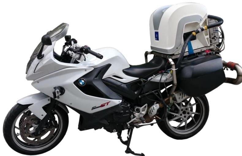
Figure 15. Full RDE measurement set up on a BMW F800GT motorcycle.
