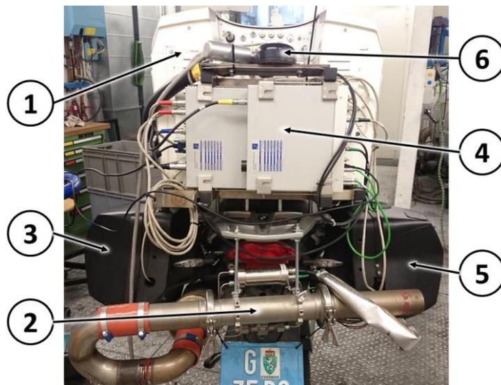
Figure 16. Measurement configuration for RDE and GPS data collection on a BMW F800GT.
