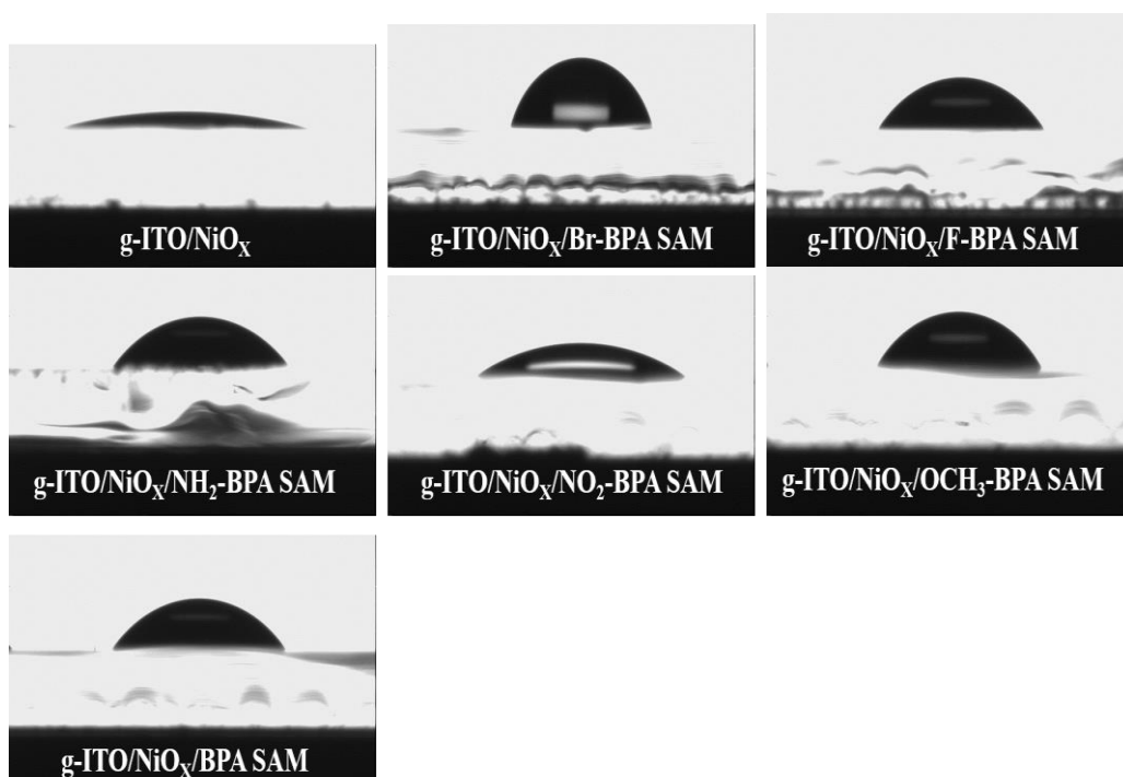
Figure 29: Images of water drops on \text{NiO}_x nanoparticles based thin films modified by dip coated R-BPA molecules.
