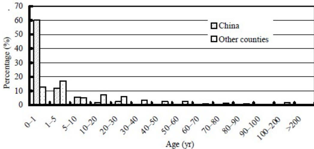
Figure 3. 17: Dam failure for different service age. China and the world (X.Y He et al, 2008)
