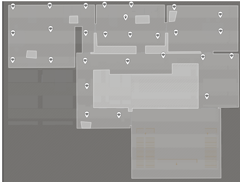
Figure 3.1: Map of the reference environment. The dark gray area depicts outside walls, the light gray area depicts inside walls/objects and the medium gray area depicts walkable space. The icons represent the locations of BLE beacons. The origin 0,0 is in the left upper corner. The x coordinate runs horizontally and the y coordinate vertically.
