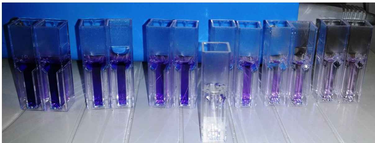
Figure 2: Preparation of calibration curve with several concentrations of glucose, fabricated in duplicates. High to low concentrations of glucose in the sequence from left to right, the blank is located in front of these samples.
