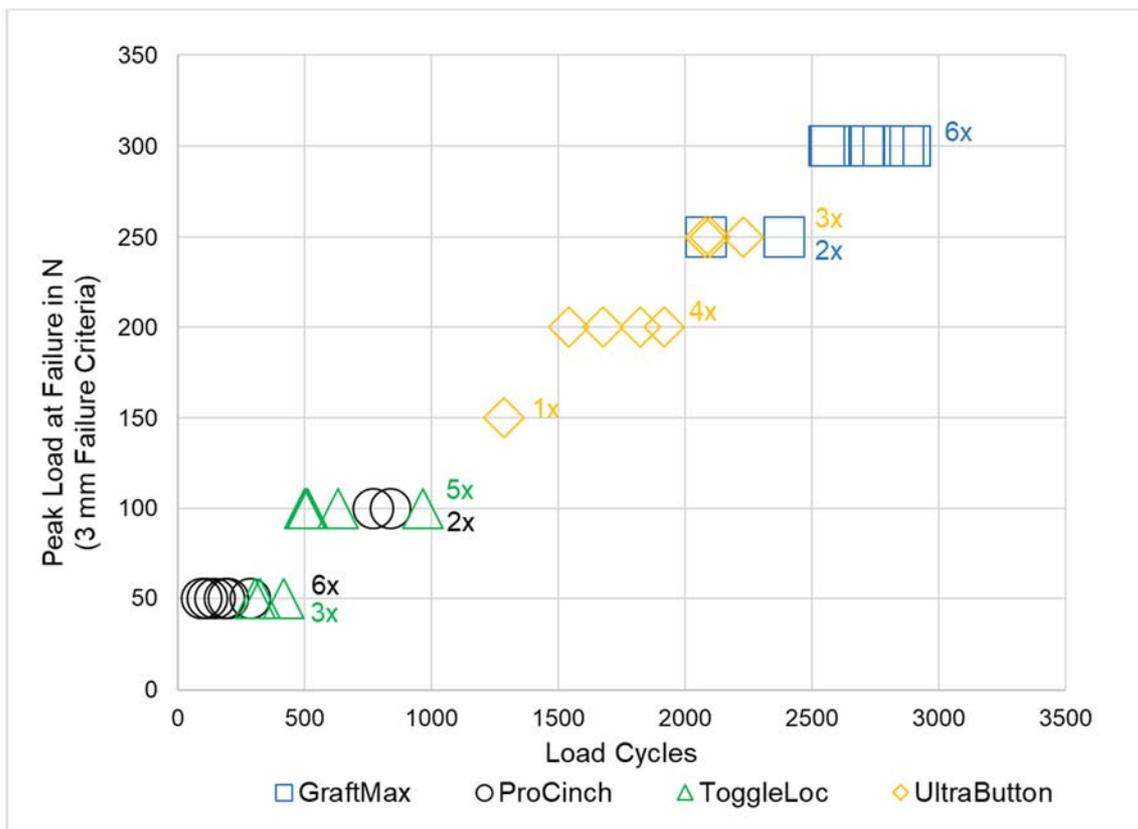
**Figure 43:** Peak load at clinical failure as a function of the tested cycles. The results of *GraftMax*, *ProCinch*, *ToggleLoc* and *UltraButton* of the single device test are shown.
