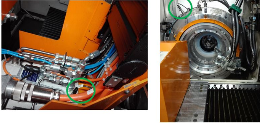
Figure 6.8: The installed sensors, marked in green, on the left on the workpiece and right on the honing ring axis
