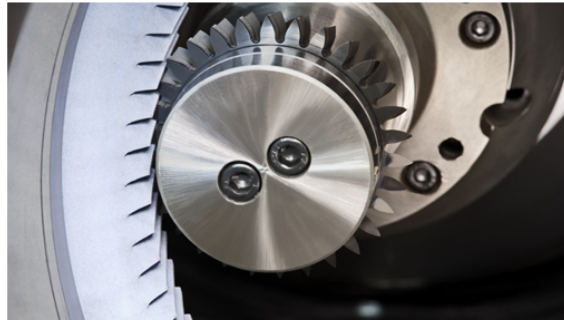
Figure 6.4: The dressing of the honing ring with a VSD (DVS Tooling, 2019)
