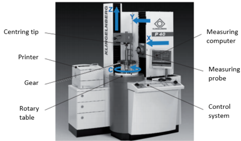
Figure 6.5: A Klingelberg gearing measurement centre (Klocke et al., 2016, pp.285)
